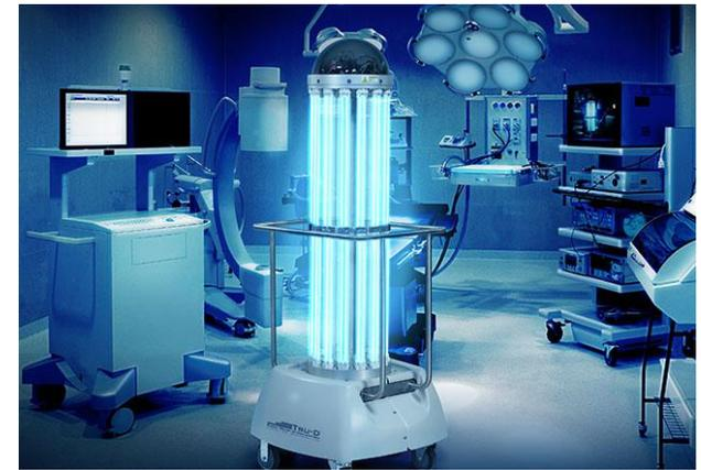
TRU-D is an automated, remotely operated, mobile disinfection system that self-adjusts to the size and content dynamics of any room to deliver an ideal lethal dose of germicidal UVC light to surfaces and air.
